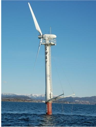
Figure 1.6: The SWAY 7 kW prototype
